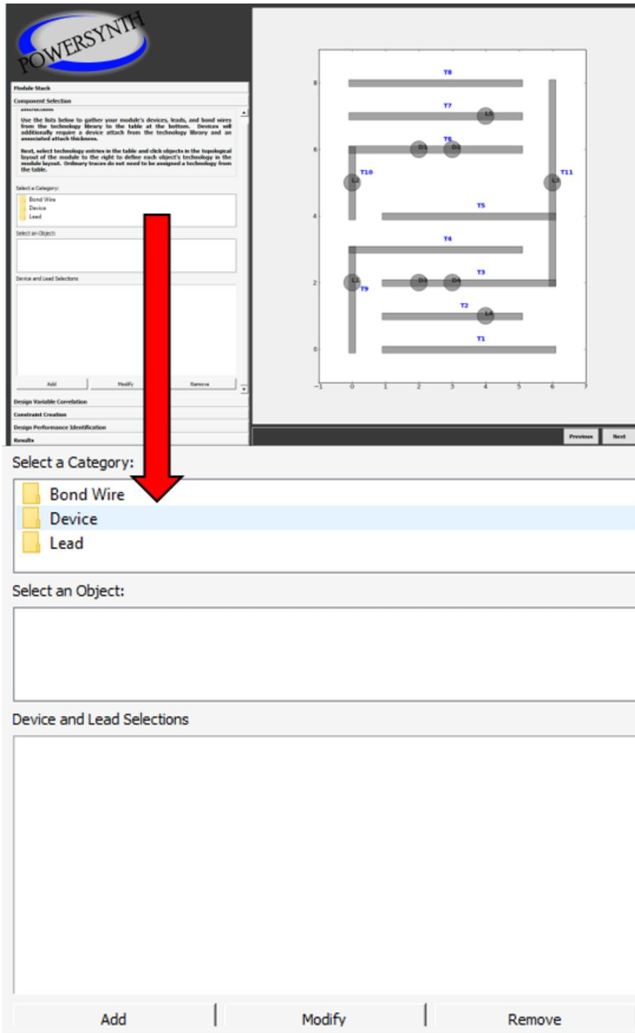
The user can assign devices and leads to the circles on the symbolic layout. The unassigned lines will represent copper or aluminum traces (depending on substrate selection). Wires bond will be treated as virtual connections. However, it is recommended to finish the devices and leads selection first before assigning virtual wire bonds to ensure correct connection.
