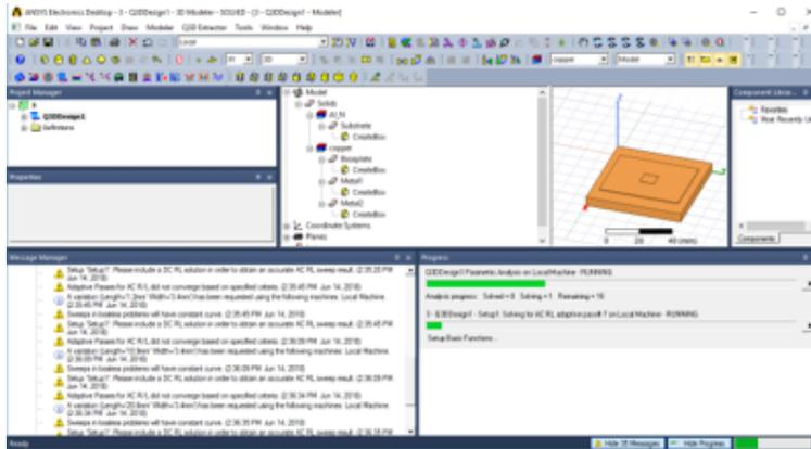
The simulation is automatically run in Q3D to characterize the model. If FastHenry simulation is selected this will be run in the back-end (Command Prompt) of the tool.
