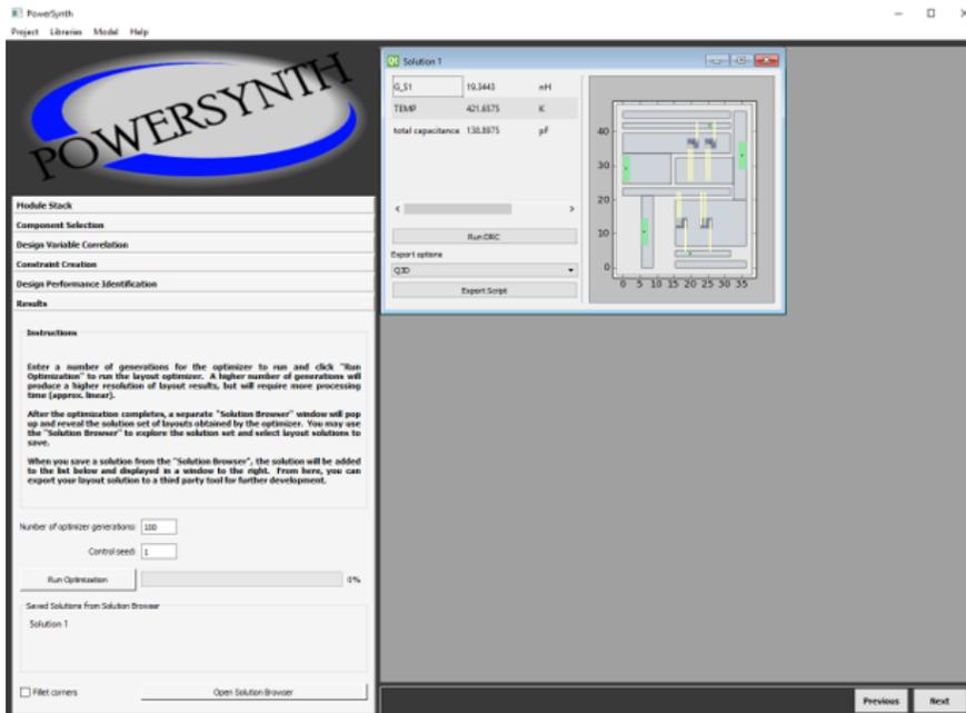
Under “Saved Solutions from Solution Browser” you can see Solution 1. The solution interface allows the user to export the solution to Q3D or SolidWorks. Other options allow the user to obtain the thermal and electrical netlists. The “Run DRC” button allow user to validate the design vs the Process Design Rule. To validate against different Process Design Rules see the section detailing the Process Design Rules Editor.
