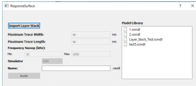
1. **Import Layer Stack:** this is explained in the Module Stack section below, this defines the baseplate and substrate dimensions. Different baseplate structures can affect the inductance calculation.
