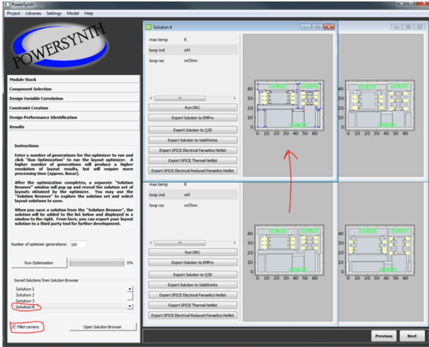
The arrow pointing up shows the same solution without fillets at the tail and with fillets at the head.
