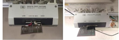
Fig. 16. Measurement setup for LR (left), C (right)
