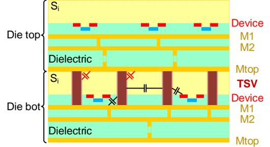
Fig. 1. Structure of 3D IC with 2 dies, the capacitance in red is the TSV-to-wire capacitance extracted in this work.
