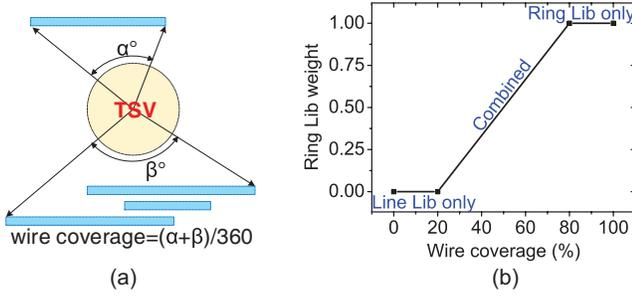
Fig. 6. Our combined method. (a) shows the calculation of wire coverage, (b) shows the calculation of weighted average.
