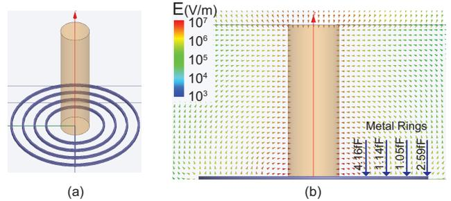
Fig. 2. Multi-wires effects. (a) TSV-ring structure. (b) E-field distribution around TSV.
