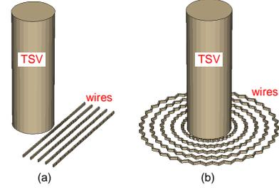
Fig. 5. Test structures for library generation. (a) Structure for line library. (b) Structure for ring library.
