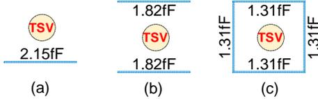
Fig. 4. Impact of wire coverage around TSV on coupling capacitance.
