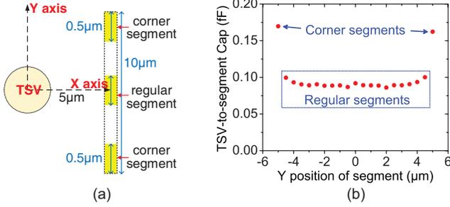
Fig. 3. Corner segment impact. (a) Simulation structure with wire segment in  $0.5\mu\text{m}$  length. (b) Extraction result for each segment.
