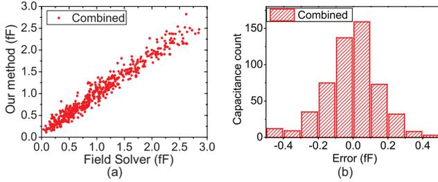
Fig. 7. Full-chip Verification using combined method. (a) shows extraction result comparison, (b) shows error histogram.
