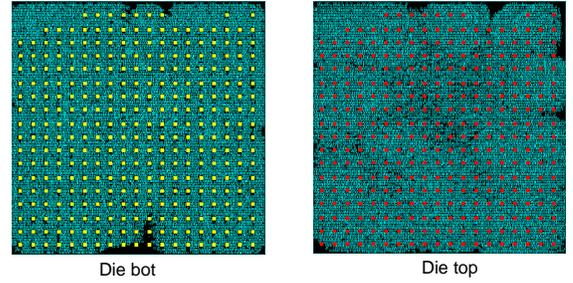
Fig. 8. Placement layout shots of FFT64. The footprint is  $380\mu\text{m} \times 380\mu\text{m}$ .
