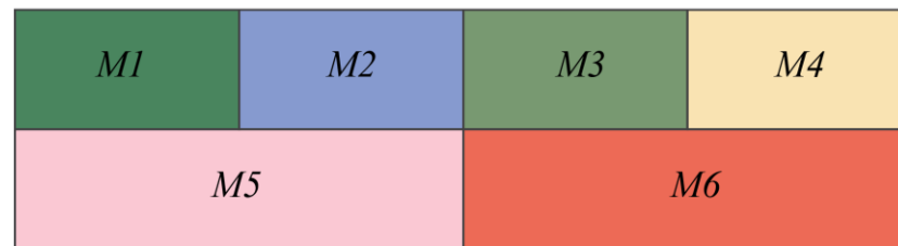
(b) Hierarchical partitioning of a 3L-ANPC inverter (a) with floorplan of switch positions (b)
