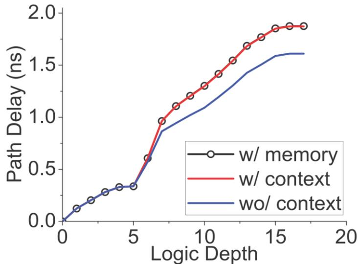
Delay propagation of the longest path
